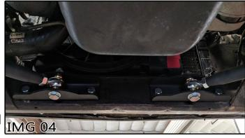
2. Bolt the new TC Rod into the TC Rod IMG 04 mount. (IMG 04)
