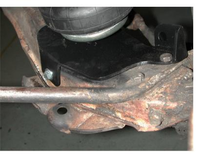
1. Place the lower air spring plate onto the lower control arm as shown in the picture. This is the driver side. The plate will index off the rear strut arm bolt. The other two holes must be drilled for 3/8" bolts.
