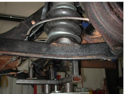
7. Bolt the lower mount to the bottom of the air spring using a 3/8" bolt. Before tightening, make sure it aligns with the lower arm.
