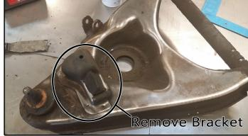
**2.** Once bump-stop bracket is removed, clean area thoroughly, as shown.
