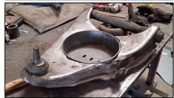
**7.** Tac the drop pocket cup into place and then weld around the perimeter as shown.
