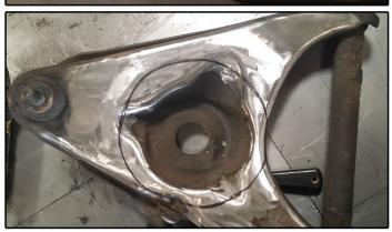
**4.** Cut inside of the traced line, and check fitment. If drop pocket cup does not fit remove more material.
