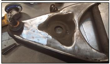
**3.** Place the drop pocket cup onto the control arm, and trace around the outside diameter with a scribe or marker.
