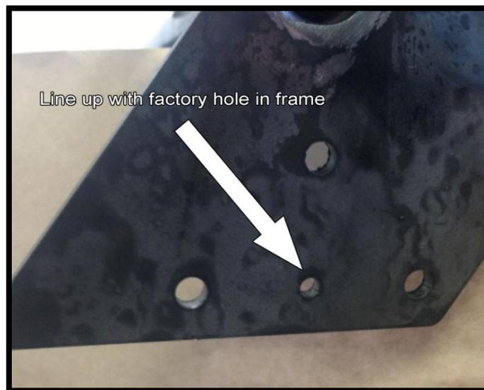
6. Mark the three additional holes to be drilled through the frame rails on each side, then remove the crossmember again. Drill these holes through the inside and outside of the frame rails with a 3/8" drill bit. Then drill JUST THE INSIDE frame rail with a 9/16" drill bit. Slide the frame sleeves inside these holes.
