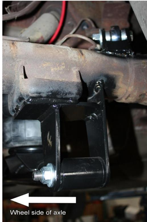
12. Swing the lower link bars up to meet the leaf spring mounting pads on the axle, and clamp the axle brackets to them. Check that the axle is centered and lined up, then tack weld the brackets to the axle to set their position.
