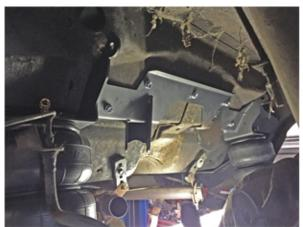
The upper crossmember can now be bolted in. It will bolt to the side brackets, then to the floor of the car. To access the inside of the panel, some years will require holes to be drilled through an inner panel. There are body plugs included with the kit to cover those up.
