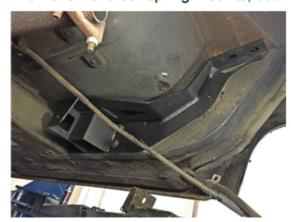
Bolt new frame brackets onto car as shown. Use the original leaf hanger mounting bolts to secure them, then use self-tapping bolts through the remaining holes into body structure.
