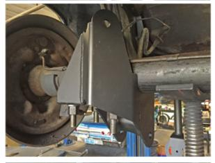
Axle brackets bolt directly where the leaf springs used to go as shown. Use the U-bolts included in the kit. Be sure to move brake lines so they don't get pinched.
