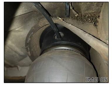
**7.** Re-check airbag fitment, RUBBING WILL RESULT IN AIRBAG FAILURE! This is a non-warrantable issue.
