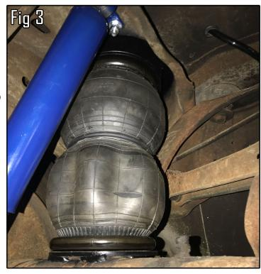
Brackets are designed for use with 6" 2500lbs or 7" 2600lbs air springs Such as Air Lift D2500/D2600 or Slam Specialties RE6/RE7.
