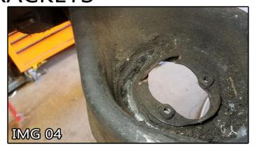
5. Remove the lower spring pocket retainer.
