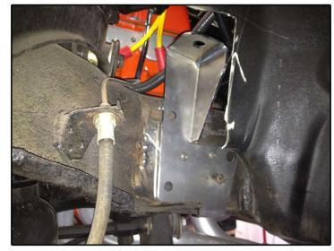
2. Mark the hole in the bottom of the frame and drill with a 5/16" bit. Use the 3/8" self-tapping bolts supplied and bolt the bracket to the frame. mark and drill the remaining holes.
