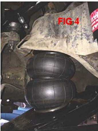
8) Upper air bag cup will need to be center into the upper coil pocket teeth. You will then use the supply flat laser tab to secure it in place. It maybe require to eliminate both upper L shape shock tabs. You can install 7" Dia air bad with no trimming. See (fig 3 & fig 4)
