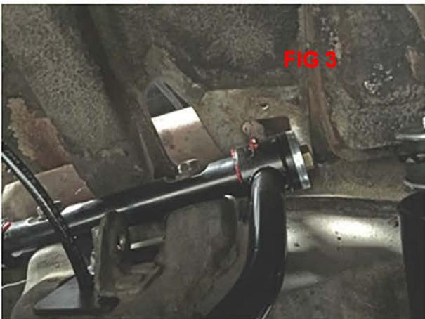
9) Upper shock towers using to factory holes. You will need to drill 3 addition holes to install. Use supplied 3/8" nut insert to install. Use drill size 17/32" (.531"). See (fig 5)
